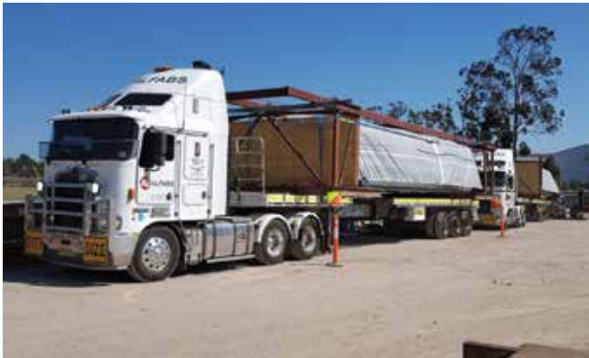
CATEGORY: Over Dimensional Transport LOAD: Roof Sections 4.5 Metres Wide
