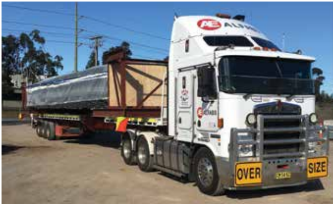
CATEGORY: Over Dimensional Transport LOAD: Roof Sections 4.5 Metres Wide
